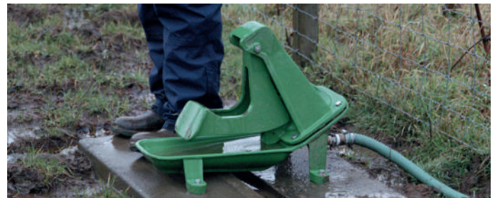
Figure 1: Pasture pump. As livestock drink from the water bowl, they push the lever to reach the water, which refills the bowl.
