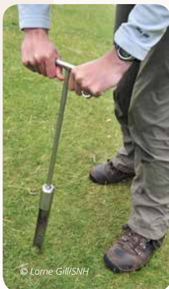
Use a soil corer or spade to take a sample
