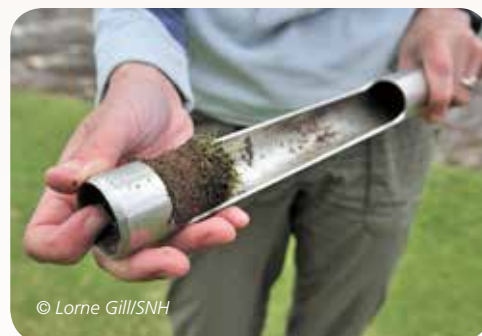
Use a soil corer or spade to take a sample
