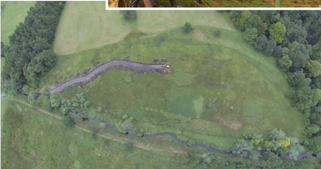
Figure 1-3 Cutting a more natural channel on the floodplain.
